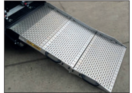
Ultra light weight ramp - gas strut assisted.
